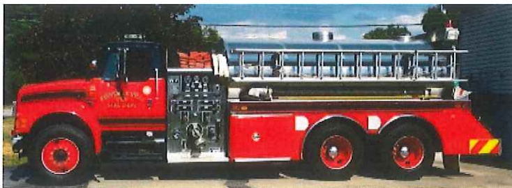
1994 Semo Tanker, 2,600 Gallons of Water, 1,250 Gallon per minute pump
